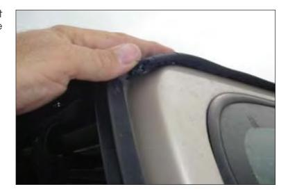
6. Lay fabric top over frame and orient it on vehicle. Snap fabric to middle and rear bows.
