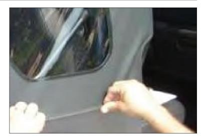
14. Push inner spreader bars up until they snap into place.
