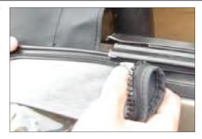
16. Fasten snaps on soft top, above doors, to studs on vehicle. Studs slide to match location of snaps on soft top.
