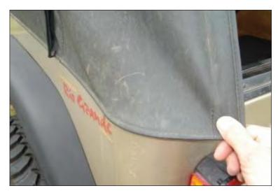
5. Unsnap soft top from above doors, remove front plastic strip from windshield channel, and remove soft top fabric.
