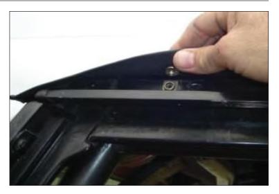
17. Remove fabric upper doors from vehicle. Using razor blade, cut stitching on old door covers and remove from frame.
