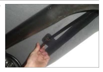
15. Install tailgate bar in receiver on each side of tailgate opening and slide rear window into tailgate bar. Start zipper of rear window. Hold up window and finish zipping rear window to top.
