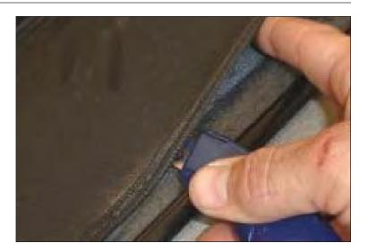
18. Separate hook and loop fasteners on new door skins. Lay door skin on flat surface with outside facing down. Start by working lower rear corner of door frame into pocket in lower rear corner of door skin. Continue working door skin around frame and fasten hook and loop strips as you go.
