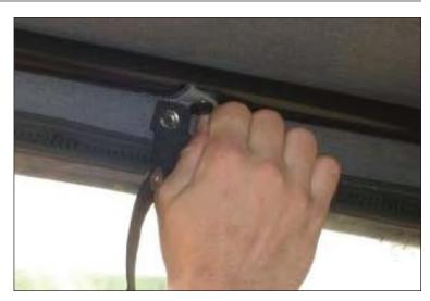
3. Pull down on spreader bars and push rear support bow forward.
