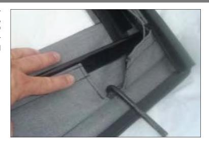
19. Reinstall upper doors. Insert pins into grommets in lower doors. Fasten snap at front of upper door. Slip plastic strip on bottom of door skin into retainer on lower door.
