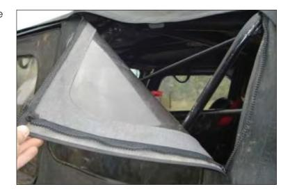
12. Slide plastic strip on front of side window into retainer channel on front support bow.
