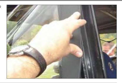
13. Slide plastic strip on bottom of side window into belt rail. Start at one end of window and work along vehicle to other end. Close top and rear zippers on side windows.
